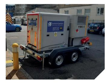
consumption and thus lower Greenhouse Gas emissions when using hybrid generators, whilst significantly reducing noise and providing better air quality for the customer. The success of the hybrid generators in BaU lead to SEPD procuring an additional 5 Hygen MX hybrid generators in November 2020.
