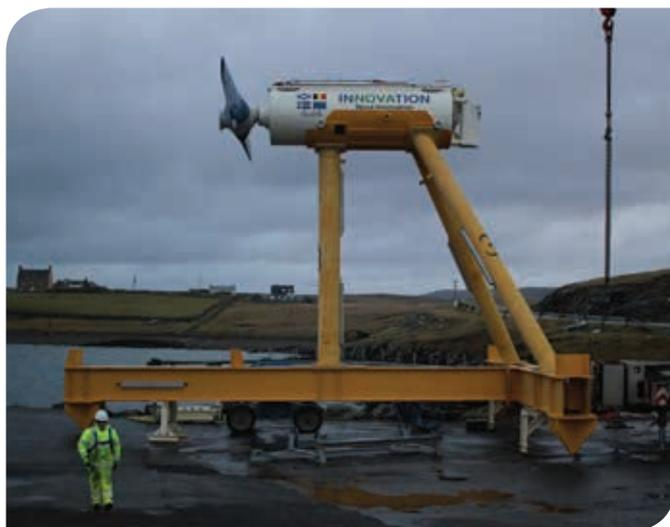
The picture above shows a tidal generator in the docks ready to be installed as part of the NiNES ANM scheme in Shetland.
