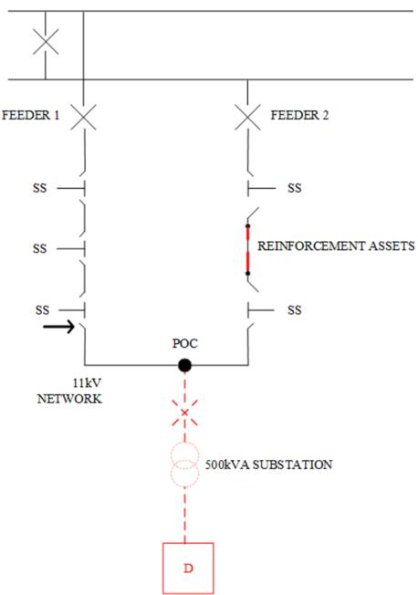
The Relevant Section of Network is the two-feeder ring comprising Feeder 1 and Feeder 2.
