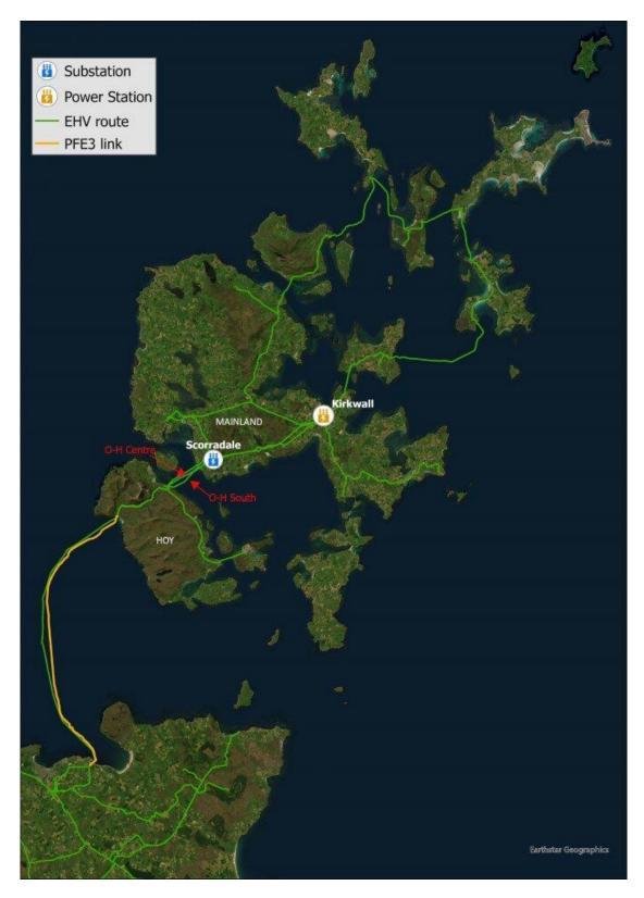
Figure 3: Existing 33kV network supplying Orkney
