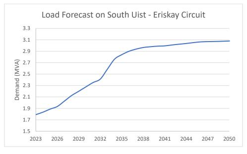
Figure 3: Load Forecast South Uist - Eriskay - 11 kV Feeder
