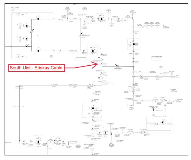
Figure 2: South Uist – Eriskay 11 kV subsea cable and network arrangement
