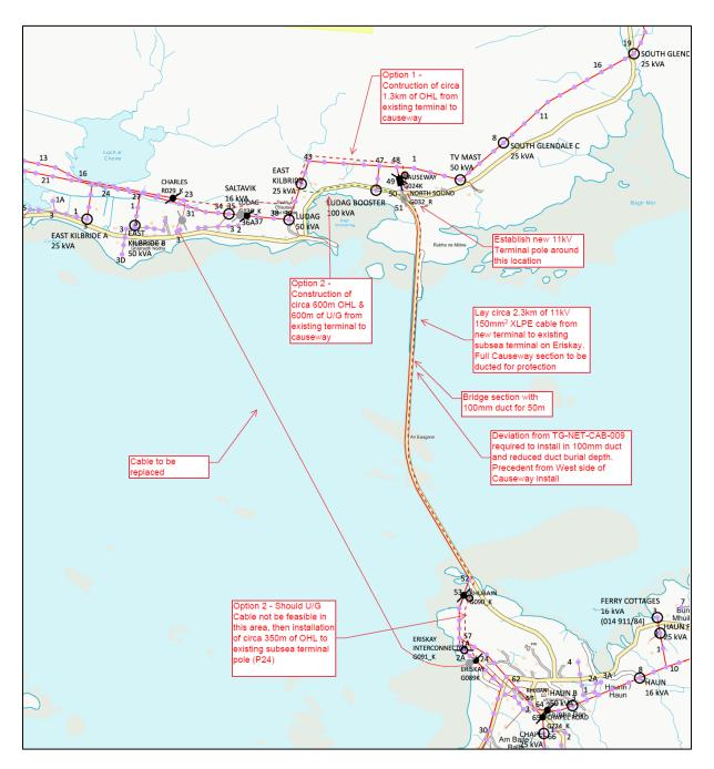
Figure 4: Proposed land-based solution for cable replacement.
