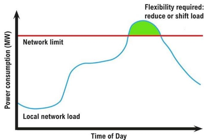
Figure 2-1: Illustration of required flexibility to reduce or shift load to stay within the network limit (Source: NEA<sup>1</sup>)
