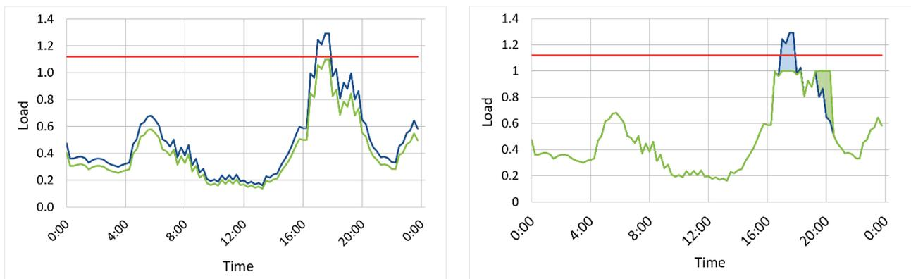
*Figure 2-2: Examples of load reduction (left panel) through energy saving and load shifting (right panel) through demand response. Without community flex the load would temporary exceed the network limits. The expected load without any measures (blue lines) is adjusted using Community Flex to stay within the network limits (green lines).*
