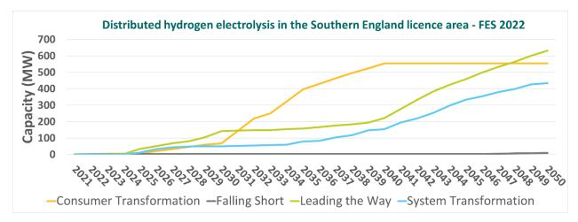
Figure 18: FES 2022 projections for distribution network connected hydrogen electrolysis in Southern England Source: FES 2022 data workbook
