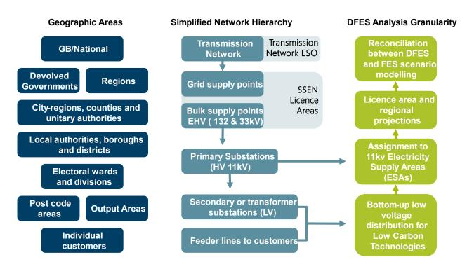
Figure 19 Network hierarchy (and associated geographic area) that determines the DFES analysis granularity for the spatial distribution to ESA
