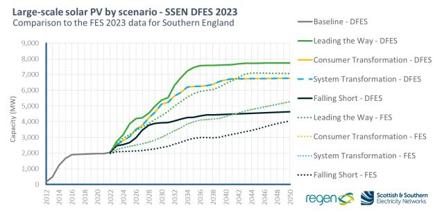
Figure 22 Large scale solar PV projections for the Southern England licence area, compared to National Grid FES 2023 regional projections. Note: Consumer Transformation and System Transformation projections are equal within the FES and DFES for this technology.
