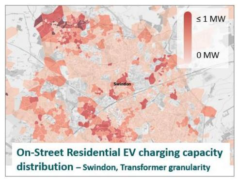
Figure 7: Transformer level geographic distribution of on-street residential EV charger capacity (MW) in Swindon in 2050, under the Consumer Transformation scenario
