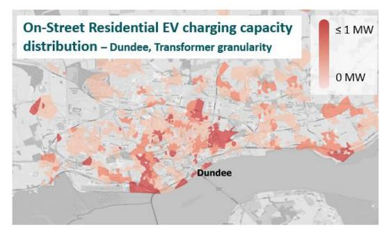
Figure 8: Transformer level geographic distribution of on-street residential EV charger capacity (MW) in Dundee in 2050, under the Consumer Transformation scenario
