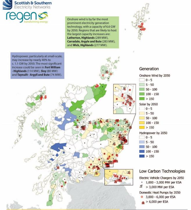
Solar capacity is concentrated in the south of the licnece area due to higher solar irradience levels and proximity to demand sources. However, as costs continue to fall and technologies efficiency improves, areas with lower solar irradience could become feasable, resulting in c. 2 GW by 2050. The regions with the highest capacity are **Leoch, Angus** (69 MW) and **Milnathort, Perth and Kinross** (57 MW).
