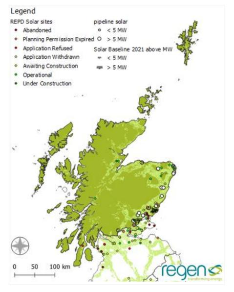
Figure 20: Baseline and pipeline of large-scale solar PV in the North of Scotland licence area, compared to Renewable Energy Planning Database
