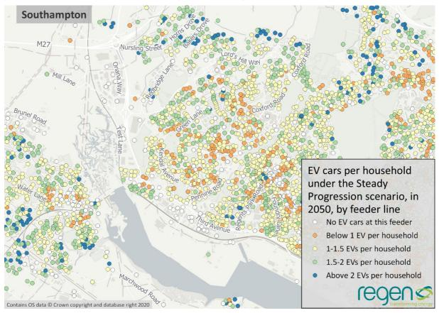
Figure 4 Electric Car distribution at feeder level in Southampton under a Steady Progression scenario
