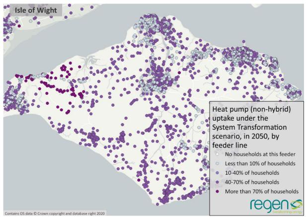
Figure 5 Heat Pump (non-hybrid) distribution on the Isle of Wight in 2050 under a System Transformation Scenario
