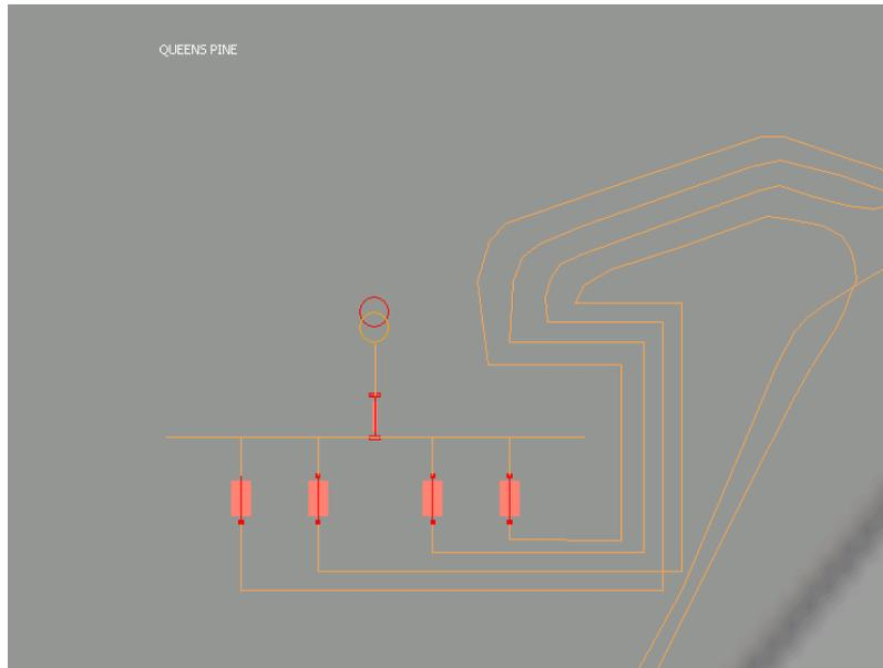
Figure 3 – 11 kV substation representation in the DMS with the secondary windings attached indicating LV network imported
