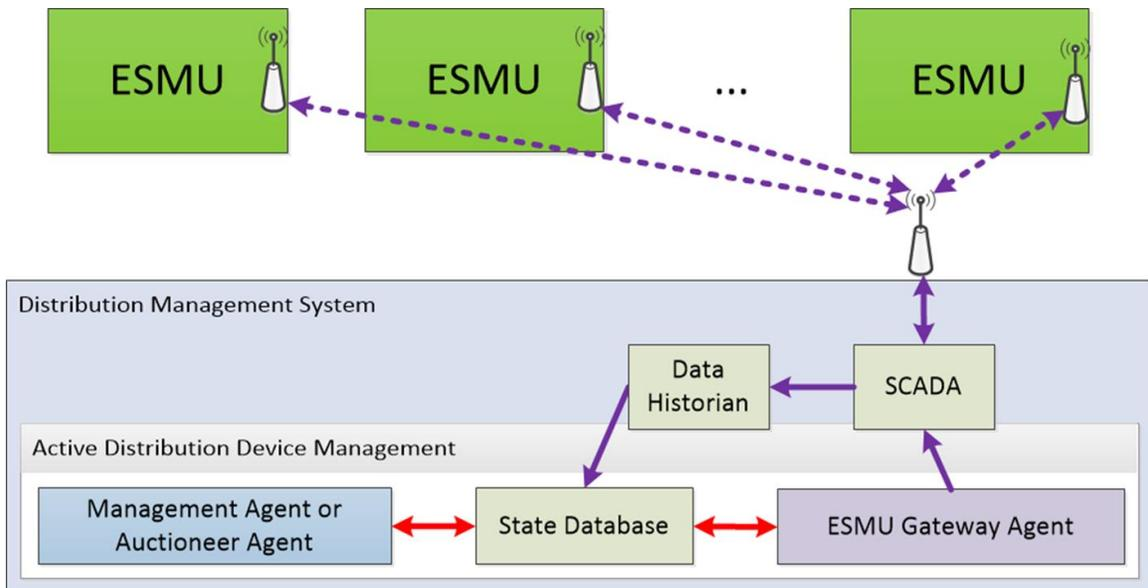
Figure 5 – High level architecture of the ADDM service and the DMS interface.
