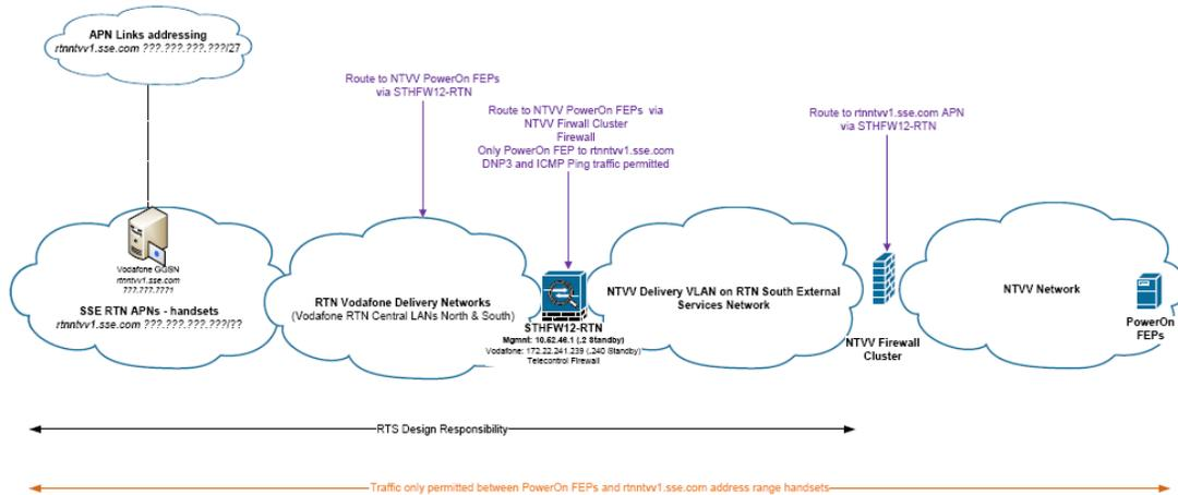
Figure 4 – Logical network design for GPRS communication to the NTVV DMS
