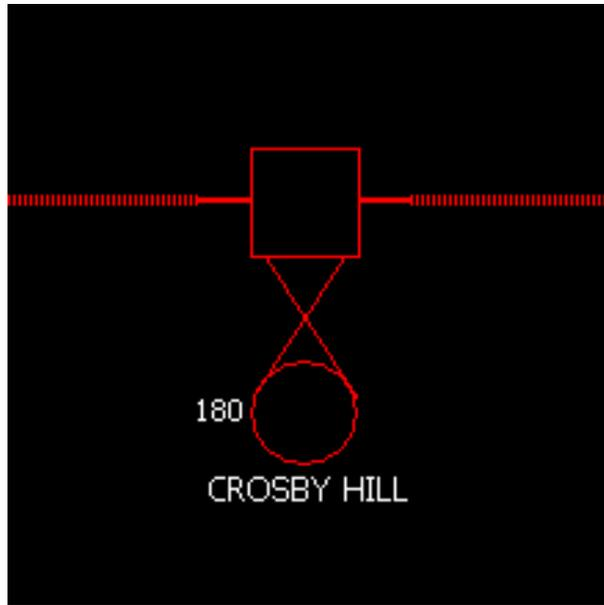
Figure 1 – 11 kV substation representation in the DMS prior to the symbol substitution
