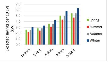
EVs represent a large amount of controllable load: an attractive option for peak reduction to network operators and customers alike, as delayed charging is normally possible while retaining convenience levels.
