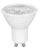
Replacing incandescent or halogen bulbs with LED bulbs can typically reduce consumption by between 80 and 90%. This can include B22 bayonet bulbs consuming 40 to 100W or GU10 or GU5.3 downlights, rated at 50W or 35W. A halogen bulb may have a lifespan of up to 2,000 hours, whereas an LED is expected to last 25,000 hours.
